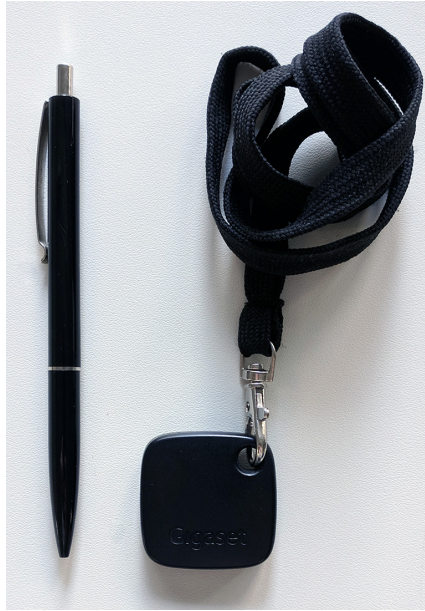
Figure 6.10: A Bluetooth Low Energy (BLE) beacon as used in the study. All participants carried the same type of beacon, allowing for a reliable detection of nearby users. Ballpoint pen for scale.
