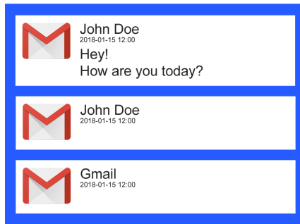
Figure 6.11: An exemplary smartphone notification mirrored to a public display. Depending on the privacy level selected by the user, the level of detail on the public display is reduced. The fourth privacy level is not to mirror notifications from the app at all. The background color (blue) is used as a color-code to provide pseudonymity.
